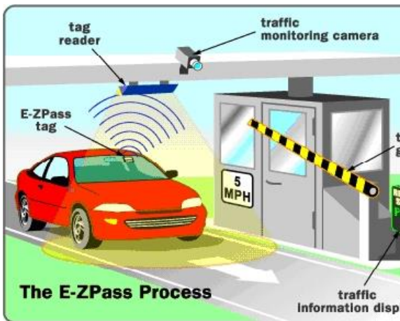
Figure 3: E-Z Pass Tolling System
